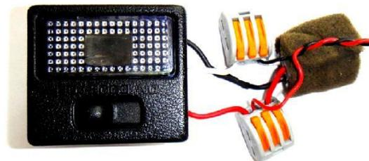
To do this, you need to cut it, isolate 3mm of its end and use the automatic connector to reconnect them and plug the third wire from the Sun Visor Light together. The connectors are having the small amber levers that will allow the cable in when lifted and strongly bite it in place when in place down.
