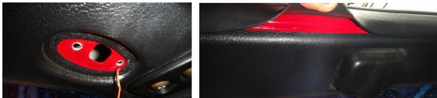
You need to guide next the cable to the cockpit. Gently pull the A pillar trim loose or to try to tap the cable behind the seal down to the hole on the side of the cockpit. You will need the cable close to the courtesy light, where it will be connected.
